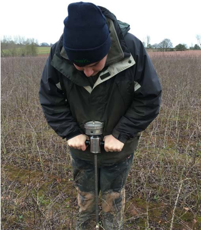
Figure 5. A penetrometer can be used to help determine the depth and extent of a compacted layer
