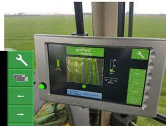
The computer continually adjusts the position of the hoe via a hydraulic sideshift or disc steer system.
